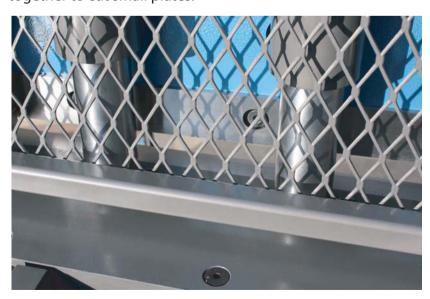
See-thru guard allows operator to see exactly where cut is being made.
